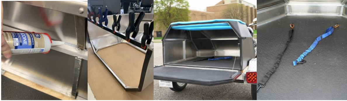
Figure 16: Assembly of the sealing and padding protection
