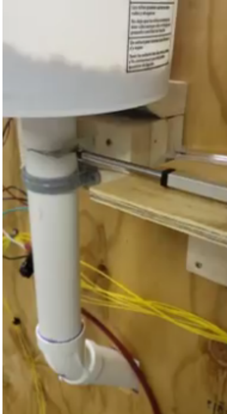
Figure 14: Feed shutoff/activation design
