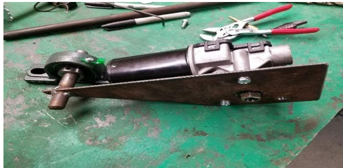
Figure 6. Motor welded on the torque arm
