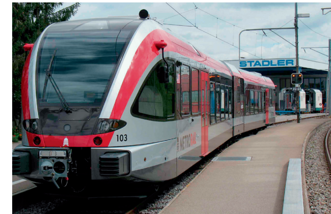
GTW DMU 216 Low-floor Light-Weight Diesel Rail Vehicle for Capital Metro, Austin, Texas, USA
